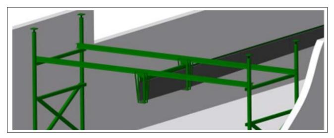
Graphic depicts a concept of how a gantry system could be installed in Room 7 to allow additional video, photographs and samples to be obtained.
